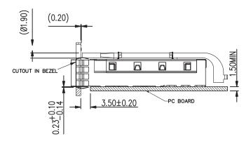
MOUNTED ON PC BOARD SHOWN THRU RECOMMEND BEZEL
