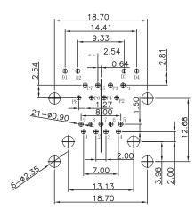
MATES WITH MODULAR PLUG CONFORMING TO FCC PART 68, SUBPART F. SUITABLE FOR CAT 5e
